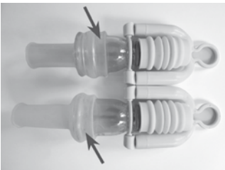
Top: Wrong, pulled too far over the bell and not powdered!
